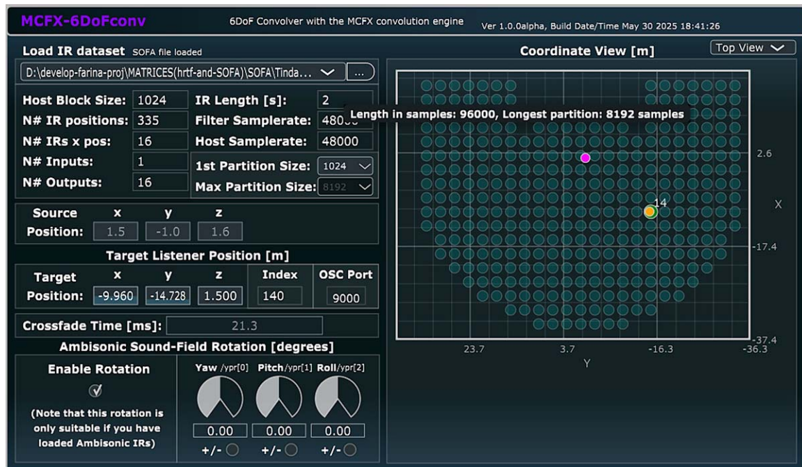
Fig. 3. Interface of the new MCFX-6DoFconv plugin. With respect to SPARTA 6DoFconv, the new plugin presents additional information displays (e.g., position crossover time in milliseconds) and controls (e.g., first and maximum partition size).
