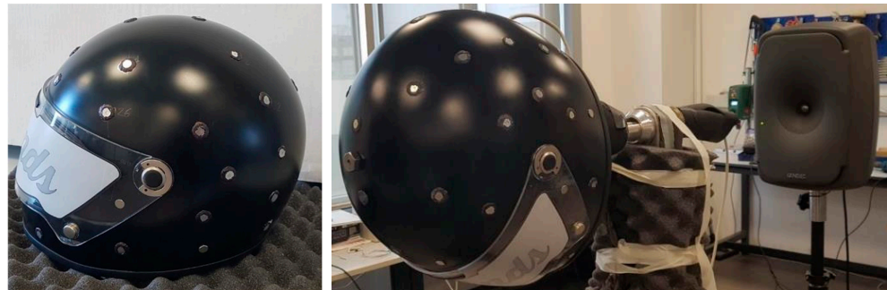
Figure 2. Side view of the array helmet after assembling the capsules ( left ). A view of the array helmet mounted on the two-axis turntable while performing the acoustic characterization ( right ).
