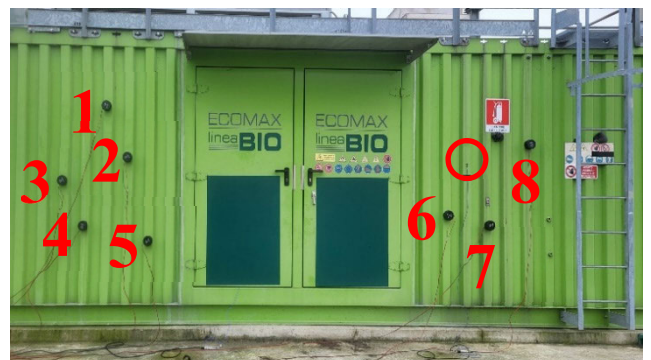
FIGURE 16. A picture of the cogenerator with the eight control shakers (numbered) and the error accelerometer (highlighted with a red circle) installed.
