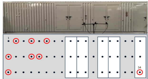
FIGURE 5. Tested cogenerator enclosure (top) and measured points with impact hammer for modal analysis (bottom). Optimal positions are highlighted with a red circle.
