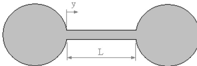
$$\vec{N}_A = \vec{J}_A = -C \cdot D_{AB} \cdot \frac{d}{dy} \left( \frac{C_A}{C} \right) = -D_{AB} \cdot \frac{dC_A}{dy}$$
