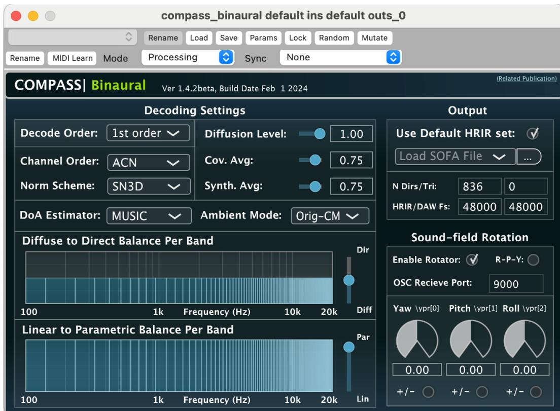
Figure 1 - Compass Binaural, a VST plugin capable of binaurally rendering Ambisonics sound-fields
