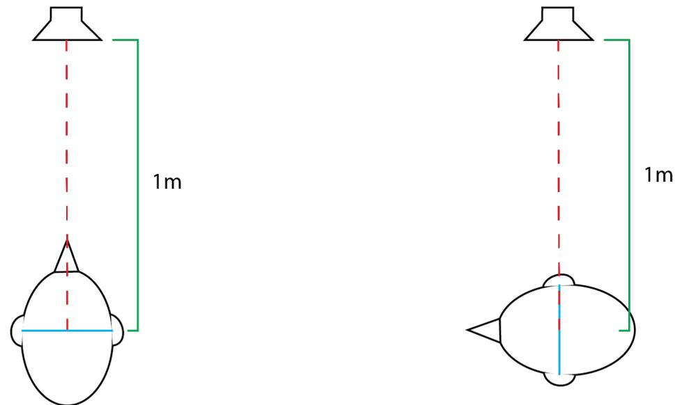
*Figure 9- Geometrical alignment of the measurements*
