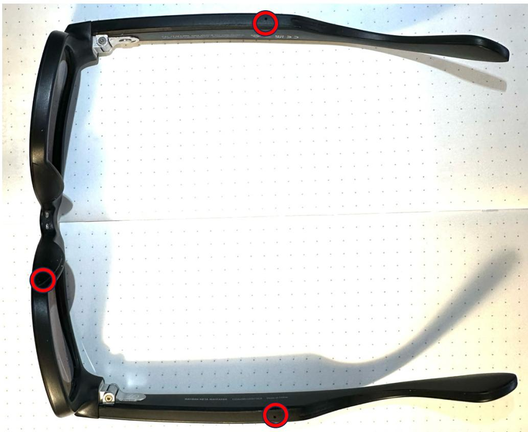
Figure 3 - Lower microphones, in the arms and near the nose pad
