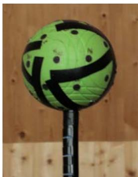
**Figure 18** 32 sensors compose the 4<sup>th</sup> order HOA microphone prototype.
