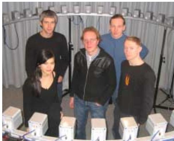
Figure 4: Listeners surrounded by a wave field synthesis array.
