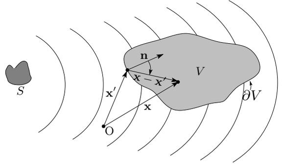
Figure 2: Reproduction of the spatial wave field emitted by the virtual source  $S$  inside the volume  $V$ .  $O$  denotes the origin of the coordinate system for the parameters of the Kirchhoff-Helmholtz integral (1).
