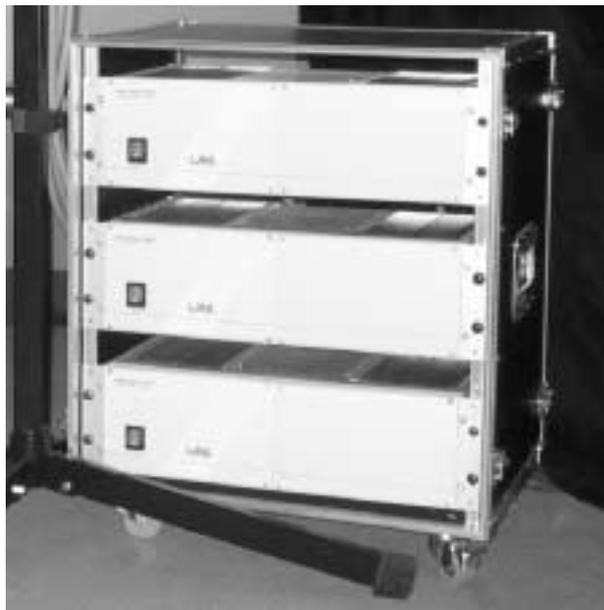
Figure 5: Three 16-channel audio amplifiers for the array in Fig. 4 mounted in a 19 inch rack.
