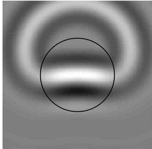
Figure 3: Reproduction of a plane wave with monopole sources. The black circle denotes a circular contour with a diameter of 3m.
