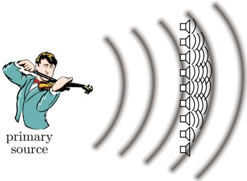
Figure 1: Synthesis of a wave front by a loudspeaker array with appropriately weighted and delayed driving signals.
