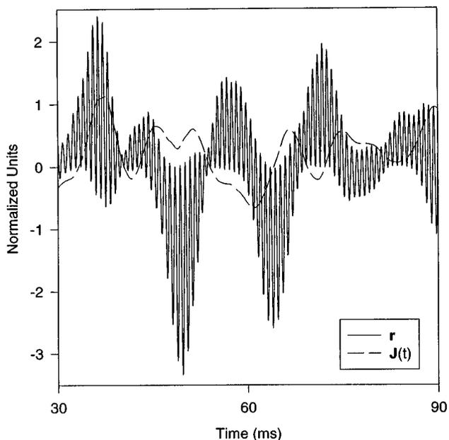
FIG. 9. Comparison of oscillating and reactive instantaneous intensities in the same field conditions as Fig. 7.
