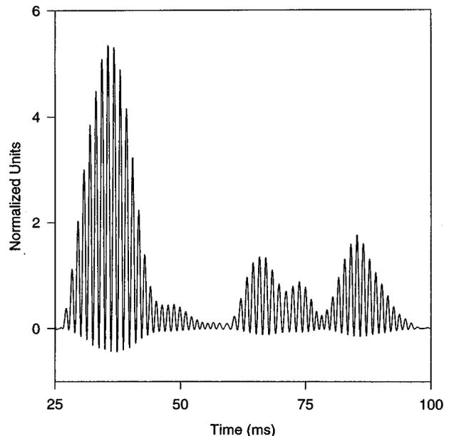
FIG. 1. Instantaneous intensity measured inside an anechoic room. Stimulus is  $\frac{1}{3}$  octave band filter noise with center frequency of 400 Hz and the distance between the loudspeaker and the facing probe is 1 m.
