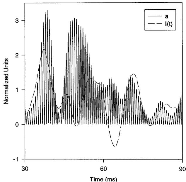
FIG. 8. Comparison of radiating and active instantaneous intensities in the same field conditions as Fig. 7.
