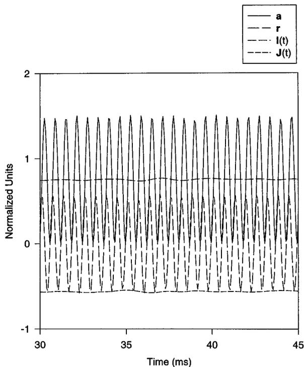
FIG. 6. Intensimetric quantities measured inside a reverberation room. Stimulus is a pure tone of 800 Hz and the distance between the loudspeaker and the facing probe is 1 m.
