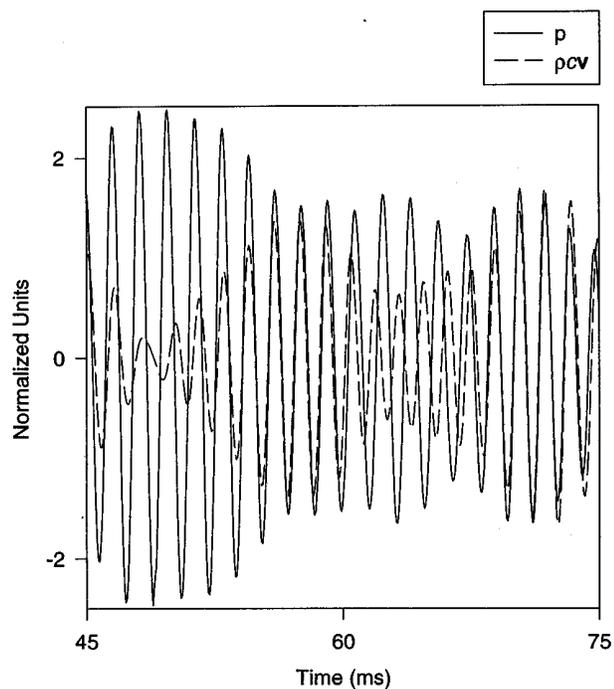
FIG. 7. Time histories comparison of pressure and normalized velocity inside a reverberation room. Stimulus is  $\frac{1}{3}$  octave band filter noise with center frequency of 630 Hz and the distance between the loudspeaker and the facing probe is 1 m.
