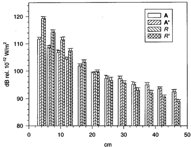
FIG. 12. Averaged intensimetric quantities measured in the region in front of a loudspeaker inside an anechoic room. Stimulus is  $\frac{1}{3}$  octave band filter noise with center frequency of 400 Hz.
