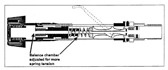
When the balance chamber adjustment is threaded inward, the tension on the demand spring is increased slightly. This position can be used to make fine adjustments which will stop a slight free-flow, following overhaul.
