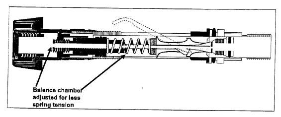
To decrease the cracking effort, the balance chamber can be threaded outward slightly, decreasing the spring tension and making the mechanism more sensitive to the movements of the diaphragm.
