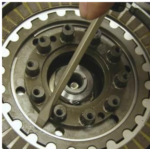
Use a screwdriver to ensure the ring is seated by sliding along the ring's inner diameter.
