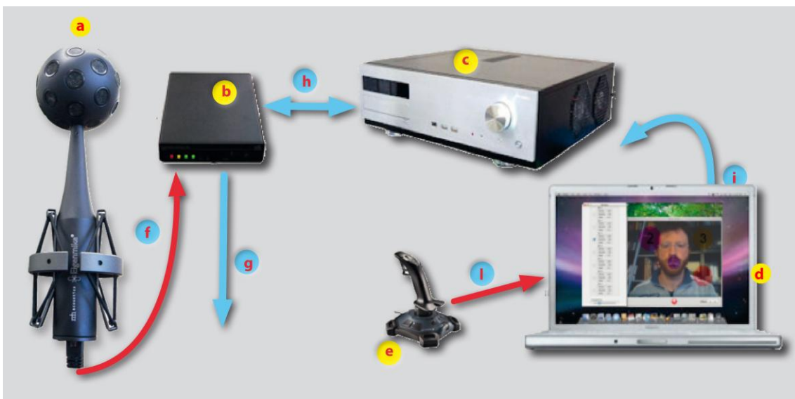
Fig. 7 – System Hardware components. a Microphone probe, b EMIB interface, c Signal processing unit, d control console (notebook), e pointing device (joystick); f CAT 6 cable, in this application it can operate up to a length of 140 m, g ADAT optical interface, h firewire interface, i Ethernet CAT 5 cable or WiFi connection, l cable or wireless connection.
