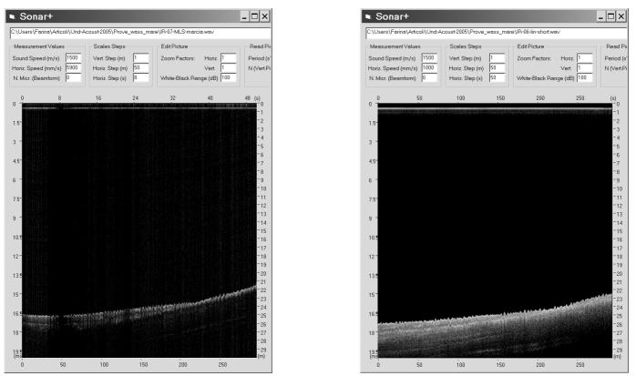
MLS (left) produces an image with lower resolution and larger noise contamination respect to "Lin" sine sweep (right).
