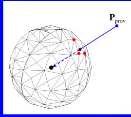
First, 4 possible nearest measurement points are located, choosing the values of  $\varphi$ and  $\theta$  which are just lower and higher than the theoretical ones.
