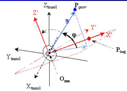
We are searching for the local arrival angles of the incoming ray: elevation ( $\phi$ ) and azimuth ( $\theta$ )
