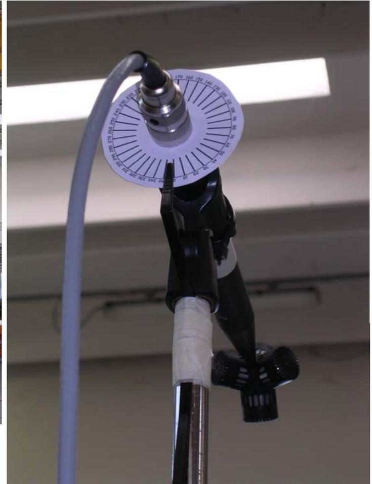
**84 IRs were measured, uniformly scattered around a sphere**
