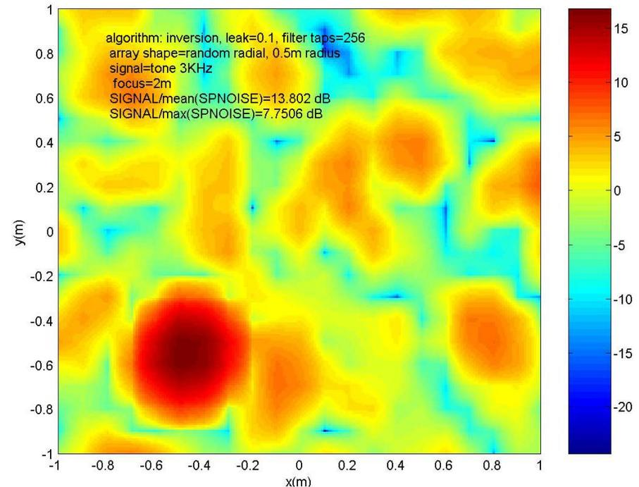
**The optimal randomized positions were found by running 10000 Matlab simulations, and choosing the one providing the better peak-to-noise ratio**
