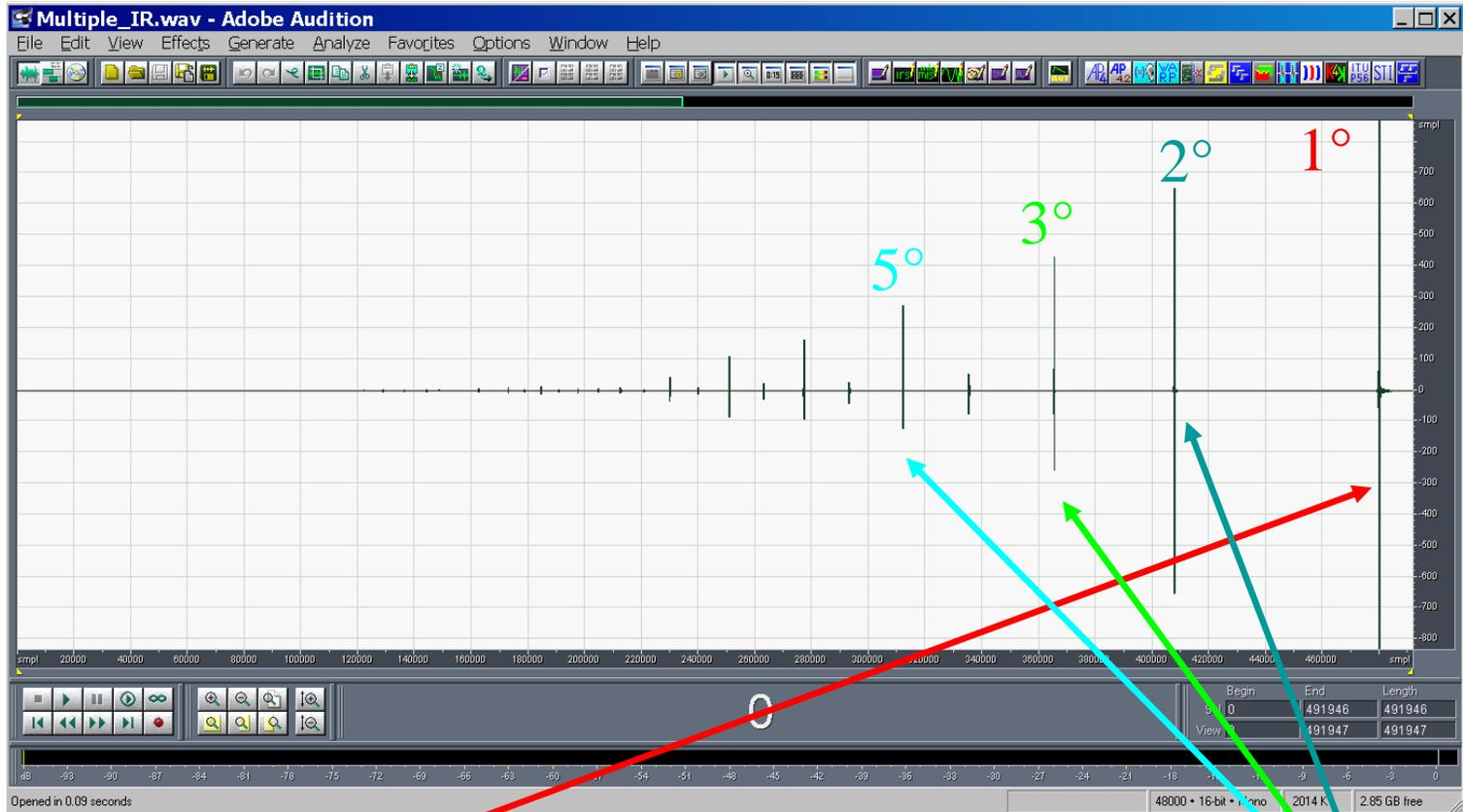
**The last** impulse response is the linear one, **the preceding** are the harmonics distortion products of various orders
