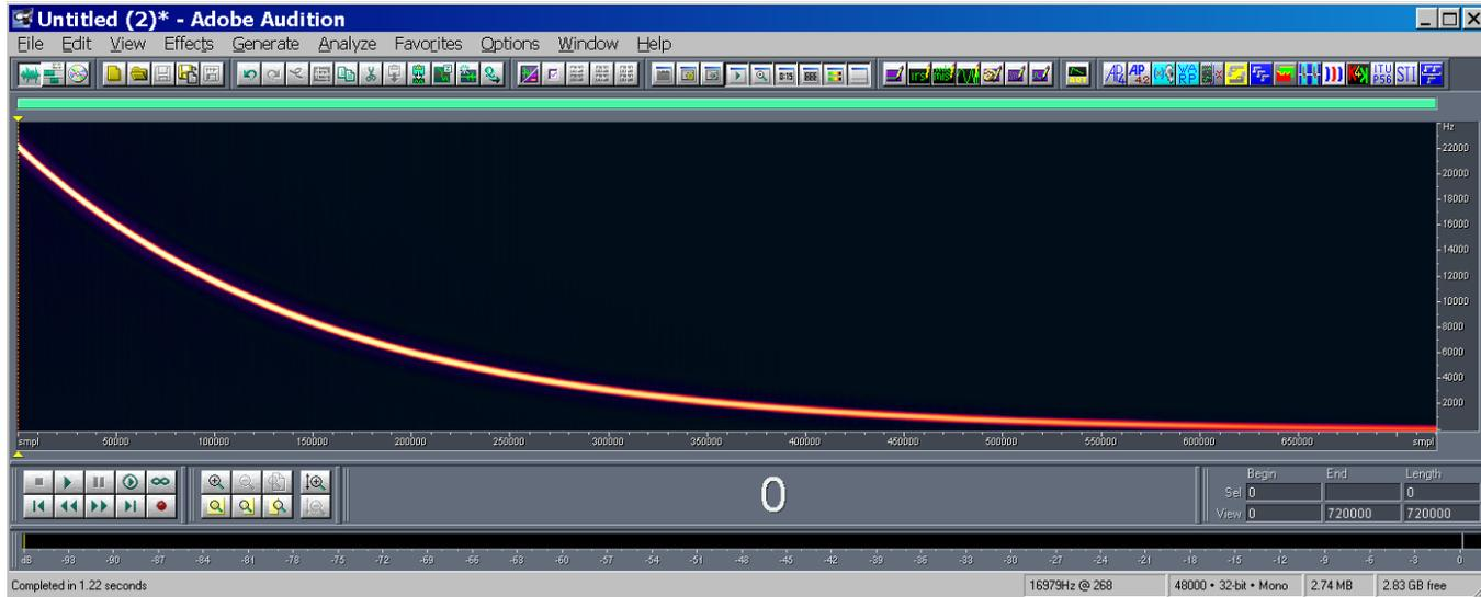
The deconvolution of the IR is obtained convolving the measured signal  $y(t)$  with the inverse filter  $z(t)$  [equalized, time-reversed  $x(t)$ ]
