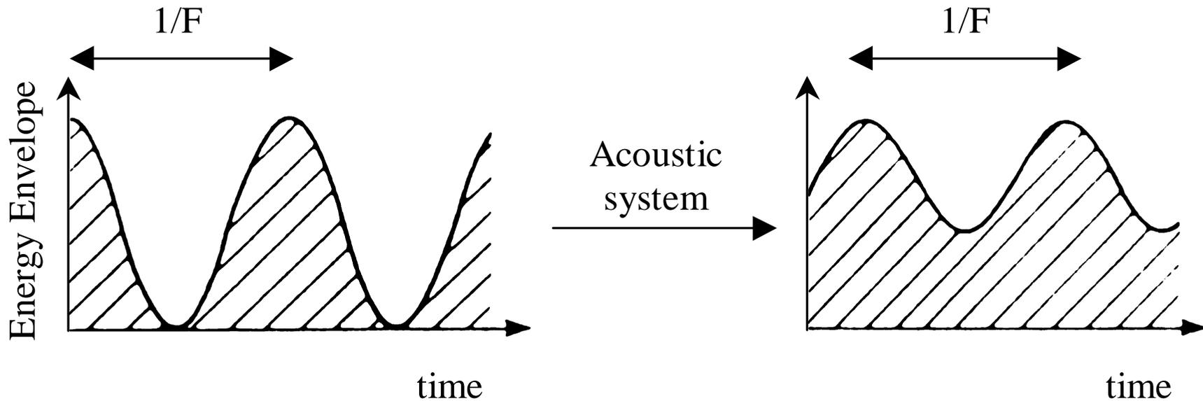
The STI method is based on the MTF concept: a carrier signal (one-octave-band-filtered noise) is amplitude modulated at a given modulation frequency with 100% modulation depth. At the receiver, the modulation depth is reduced, due to noise, reverb, echoes, etc.
