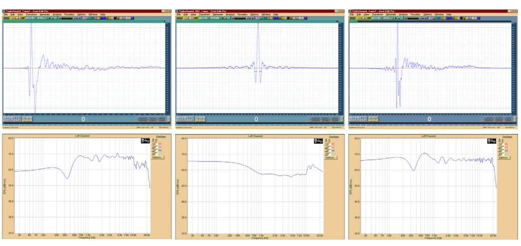
Measured transfer function of Front-Left loudspeaker Minimum-phase inverse filter (100 taps)
