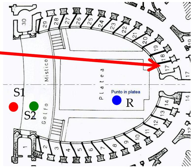
Source S2: direct sound at high frequencies is weaker than the first reflection coming after 56 ms from the proscenium arch
