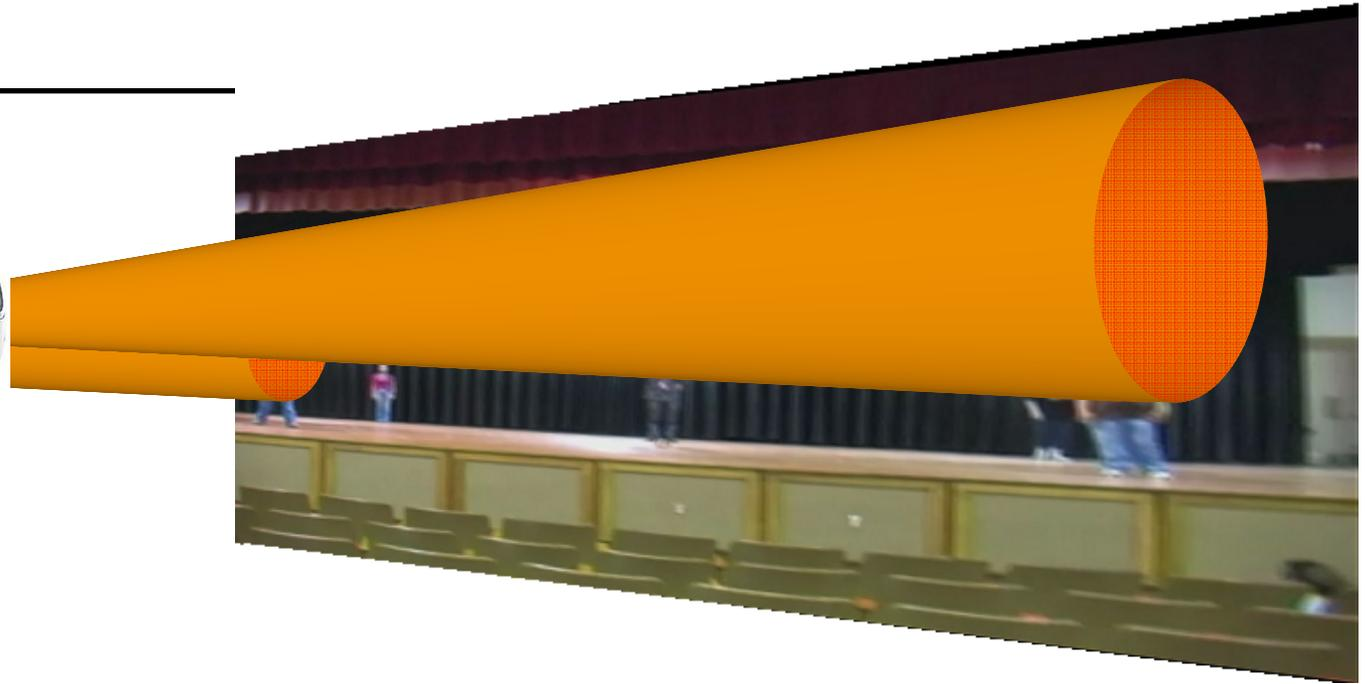
We synthesized highly directive virtual microphones starting from 32 omnidirectional ones
