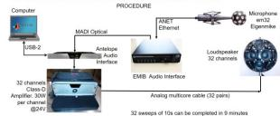
Fig. 5. Setting of the measurement chain.
