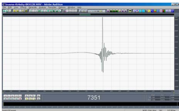
Fig. 25 – “equalizing” inverse Kirkeby filter
