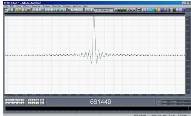
Fig. 17 – pre-ringing artifact with fade-out
