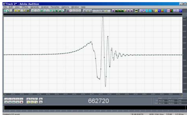
Fig. 19 – low-frequency pre-ringing artifact
