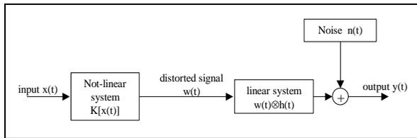
Figure 1. Flow diagram of the complex system
