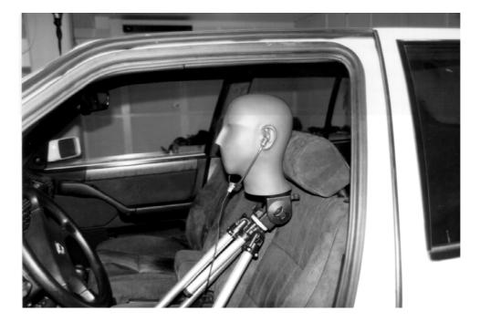
Fig. 3 – The dummy head inside a car
