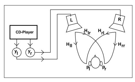
Fig. 2 - Scheme of the loudspeakers-ears transfer functions
