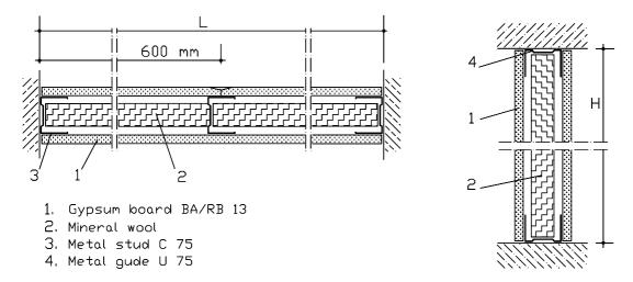
Figure 1: Horizontal and vertical sections of test specimen 1.
