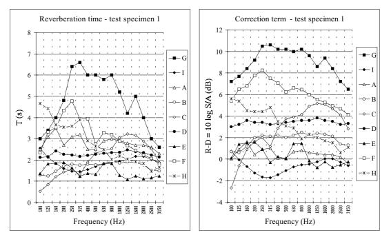
Figure 6: Reverbaration time values measured in each of the laboratories and correction term calculated to determine the sound reduction index.
