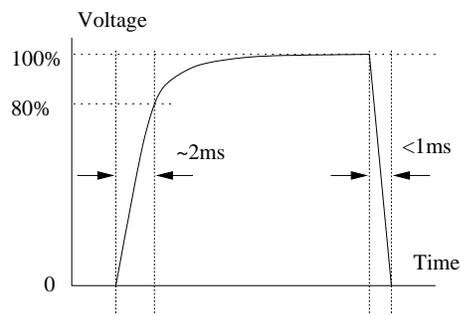
Figure 8.14: Compensated finger voltage for finger-down and finger-up.
