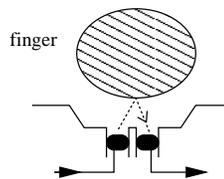
Figure 8.2: Finger proximity sensing using infrared reflection.
