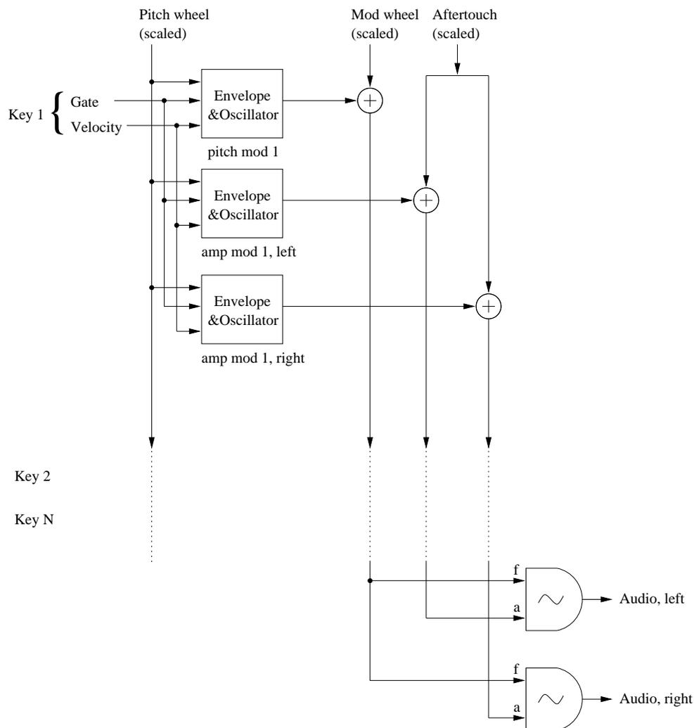
Figure 5.4: Graphical representation of Csound instrument *spiragraph2.orc*
