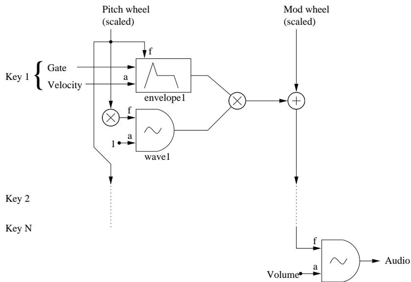
Figure 5.3: Graphical representation of Csound instrument *spiragraph1.orc*
