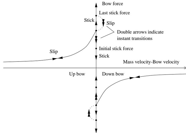
Figure 8.20: The bowforce acting on a bowed mass.
