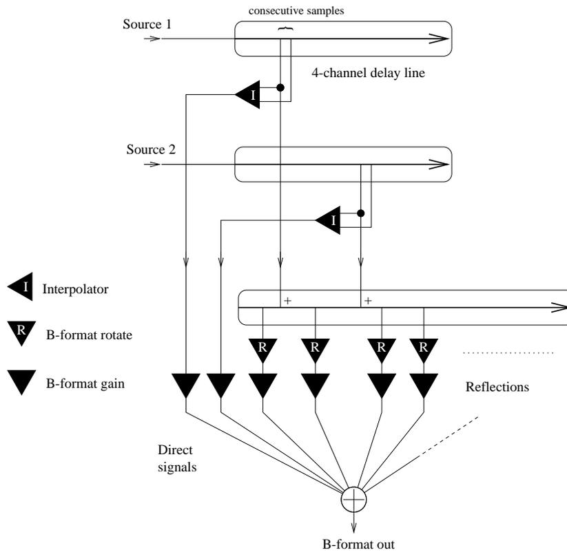
Figure 6.11: Simulating early reflections using an FIR structure.
