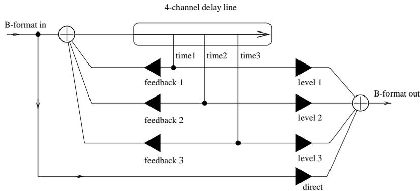
Figure 6.10: A structure for delayed feedback of B-format.
