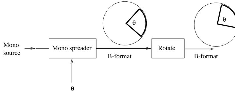
Figure 6.6: True spreader using a controlled allpass filter.
