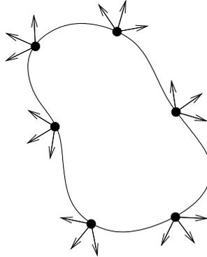
Figure 6.9: Extended surface radiator using composite point radiators.
