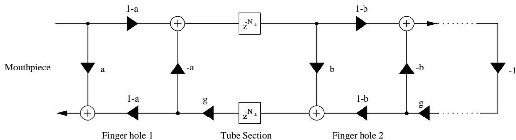
Figure 8.15: Waveguide bore model with 2 port scattering toneholes.
