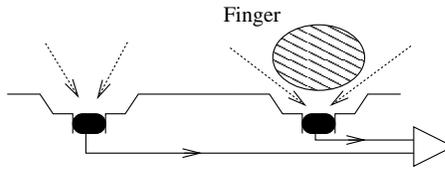
Figure 8.3: Finger proximity sensing using ambient light occlusion.
