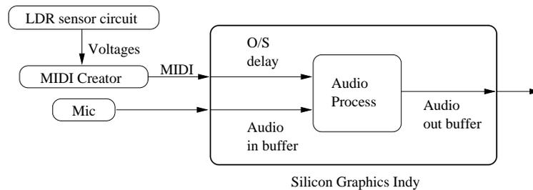
Figure 8.13: Overview of delays acting in the CyberWhistle signal path.
