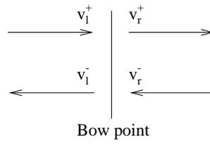
Figure 8.21: Labeling of traveling velocity waves. .
