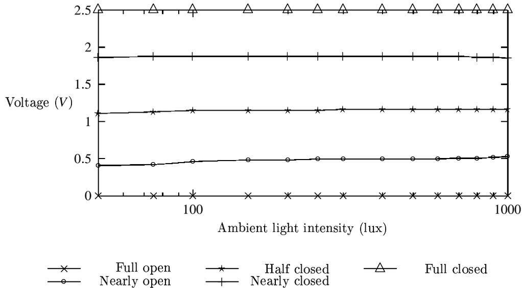
Figure 8.8: Performance test of light compensation circuit.
