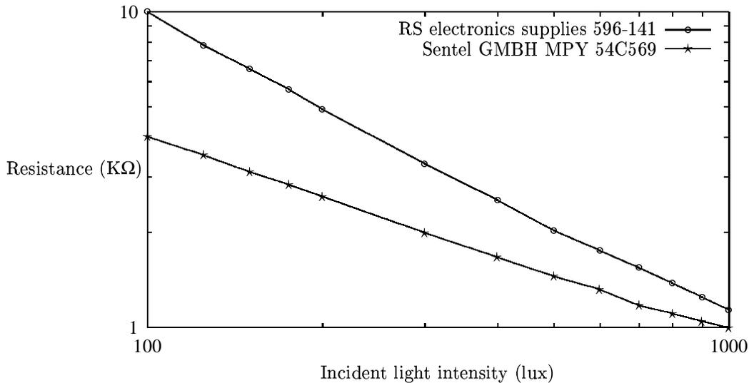
Figure 8.6: The light response of two LDRs.
