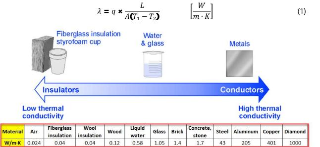
Figure 2. The thermal conductivity of common materials - describes how well the material conducts heat <sup>(3)</sup>
