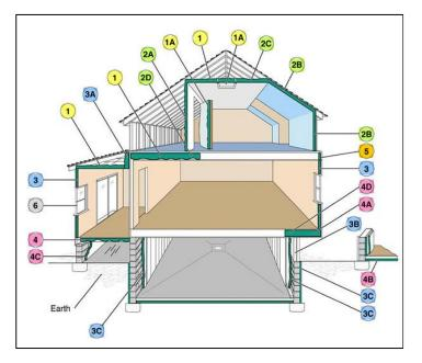
Figure 5. Examples of building insulation locations.
