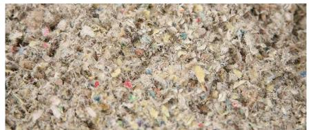
Figure 13. Cellulose Insulation.
