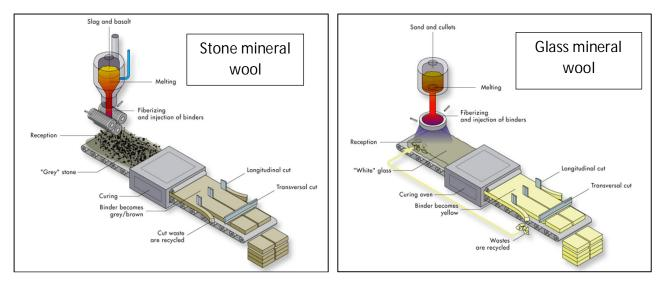
Figure 8. Production process of the mineral wool insulation <sup>(6)</sup>.
