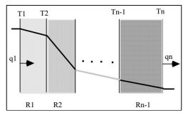
Figure 4. Heat transfer across a composite slab (series thermal resistance).
