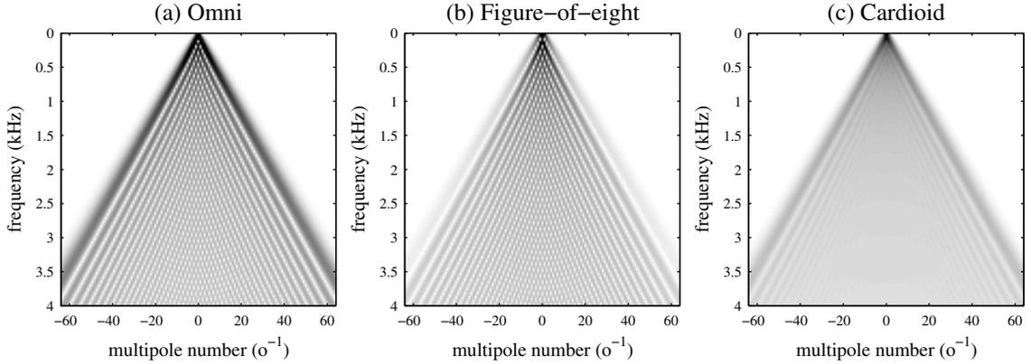
Figure 1: 2D Fourier transform of a simulated circular plane wave recording, using omni, figure-of-eight and cardioid microphones
