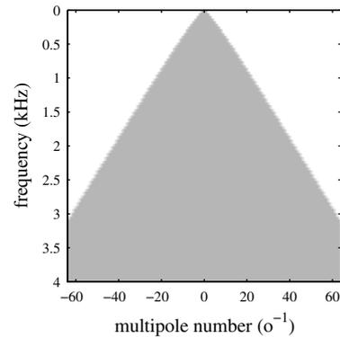
Figure 2: Cylindrical harmonics decomposition for a circular array with a 1 meter radius.
