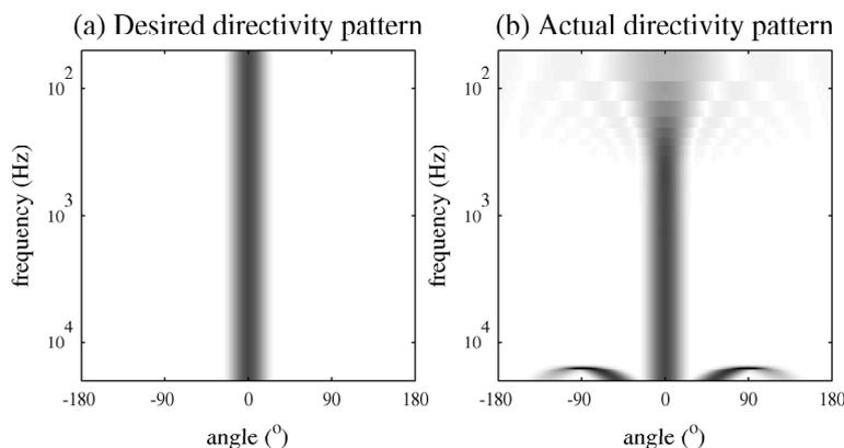
Figure 3: Directivity pattern of a virtual microphone created using a 1 meter radius array.
