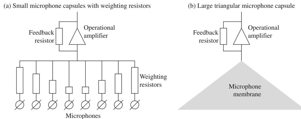
Figure 6: Panning in the analog signal domain (a) using small microphones with weighting resistor ladders, (b) using an extended microphone membrane to apply spatial weighting and integration of the sound field
