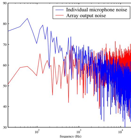
Figure 19: Noise levels from a single microphone and the complete array system
