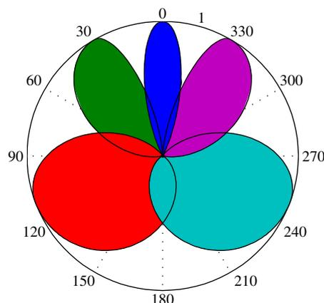
Figure 13: Desired and actual virtual microphone directivity patterns for 5.1 output using gradual panning between all 5 channels. The black lines are the desired patterns and the solid colors are the actual patterns
