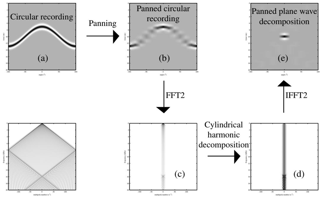
Figure 5: More efficient circular array processing for 12 virtual microphones
