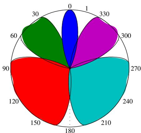
Figure 15: Desired and actual virtual microphone directivity patterns for 5.1 output using sharp transition between front and rear channels. The black lines are the desired patterns and the solid colors are the actual patterns.
