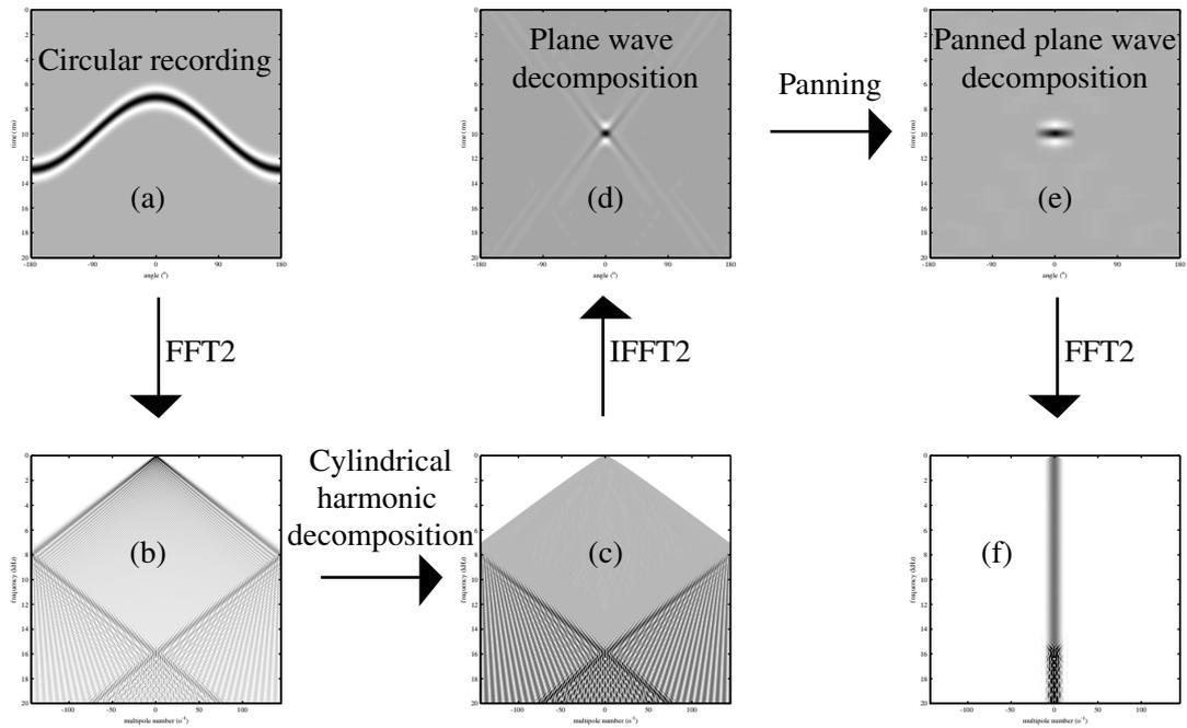
Figure 4: Circular array processing for 12 virtual microphones
