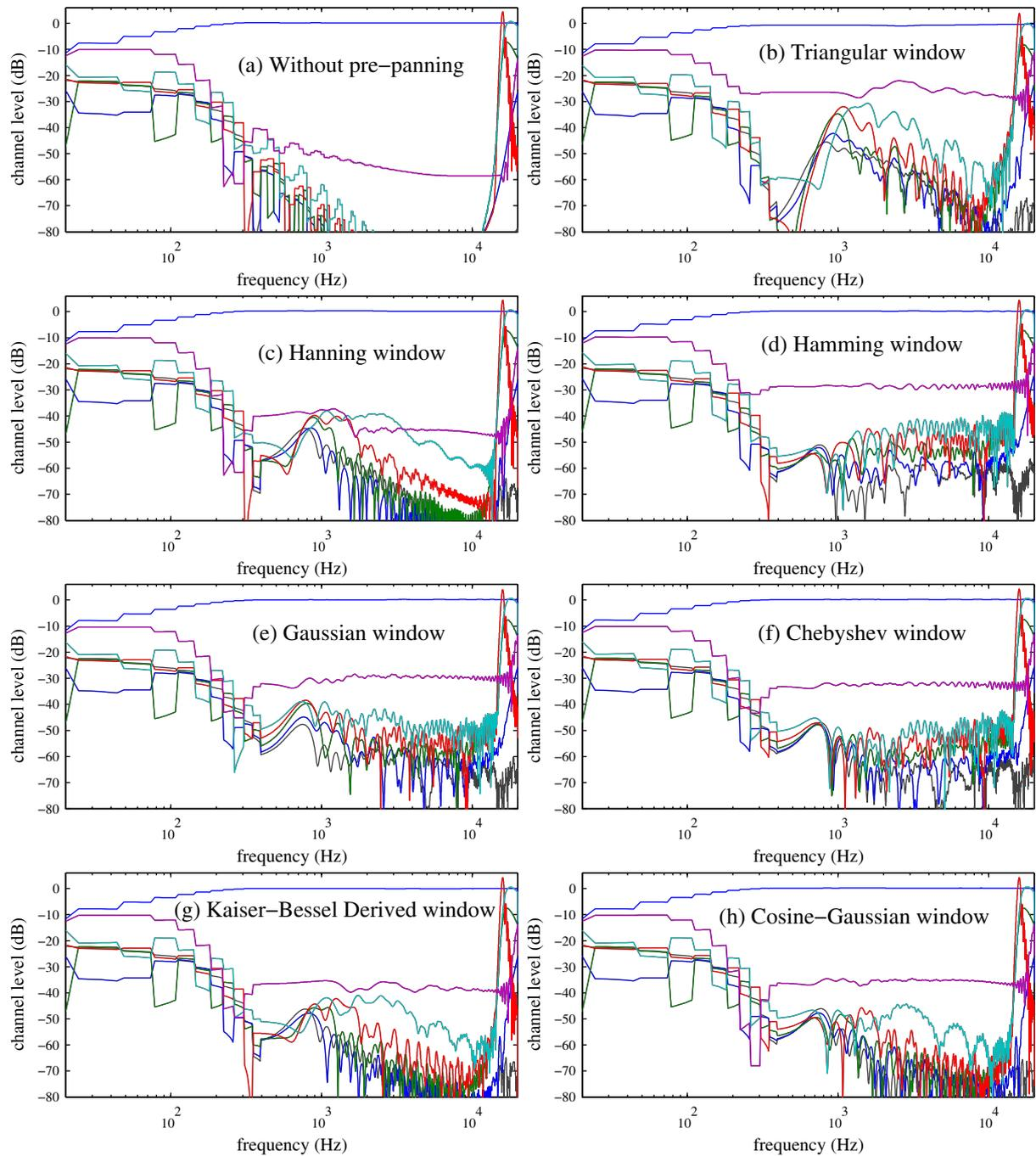
Figure 8: Aliasing performance of different panning windows recording a plane wave with 0 degree incidence, ideally being reproduced by 1 channel only
