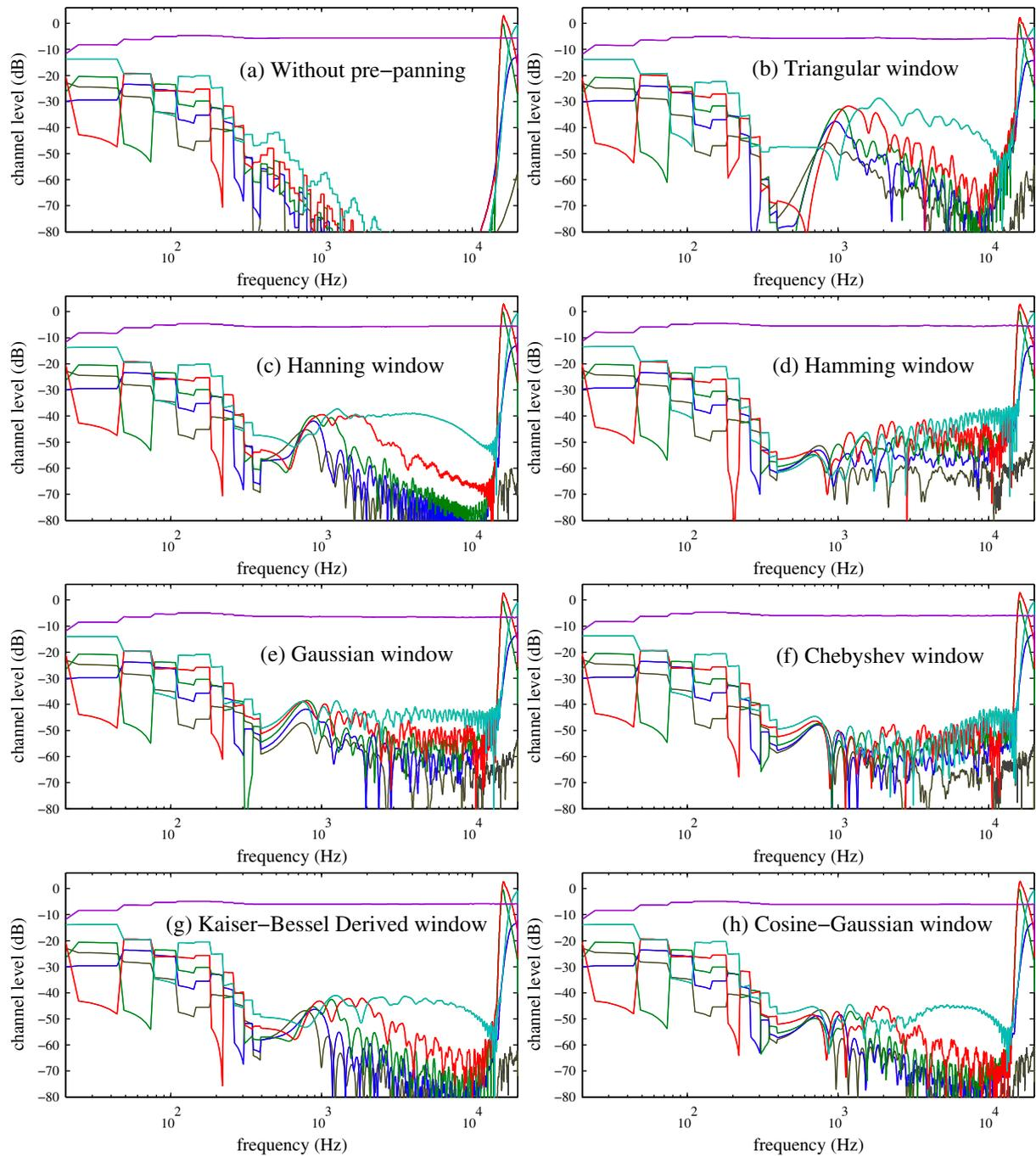
Figure 9: Aliasing performance of different panning windows recording a plane wave with 15 degree incidence, ideally being panned equally between 2 channels only
